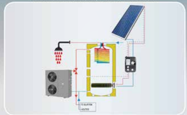
Typical Installation Buffer-1 Tank with INOX heat exchanger for Domestic Hot Water
