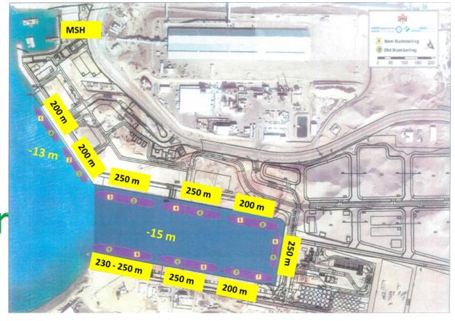
Ro-Ro: Ro-Ro vessels will be handled on berths 7, 8 and 9 as no protection curb to be installed at apron edge allowing for vessels ramp to be placed. Also the curb will be partially omitted from top of berth 6 to side more
